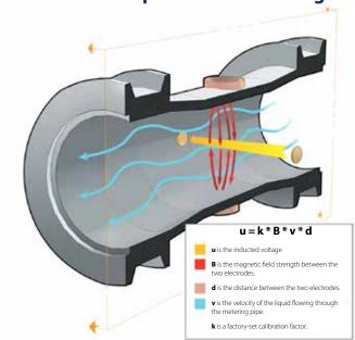
The principle of operation is based on Faraday's law of electromagnetic Induction. A highly accurate, bipolar pulse circuitry energizes two coils - creating a magnetic field perpendicular to the direction of the flow.
