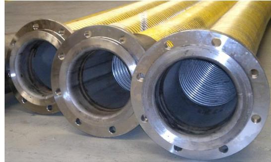
The outer cover of the Gassoflex hose is abrasion resistant PVC which protects against corrosion, attack from other liquids, UV rays and ozone. Gassoflex hoses have standard working pressures/temperatures of 10 Bar (145 PSI) to 14 Bar (203 PSI) and -20°C (-4°F) to +80°C (176°F).
